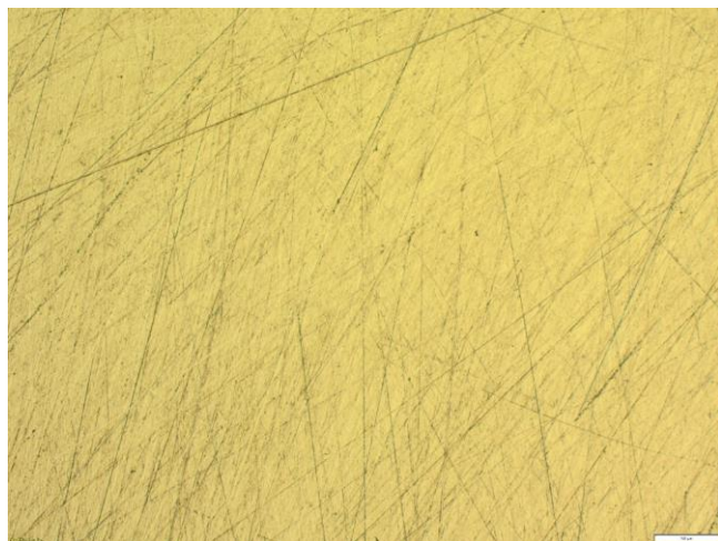
Pure MeCN, 5x No corrosion observed on coupon Solution did not discolor
