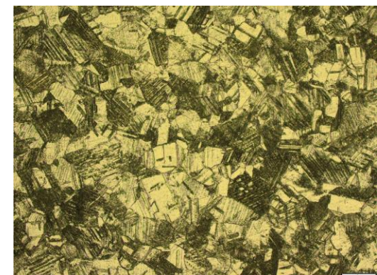
Ultimet 6B, 10x; Intergranular
