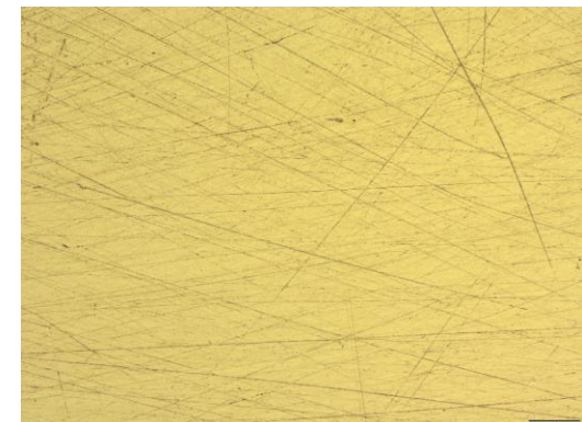
TEA, 5x; No Corrosion
