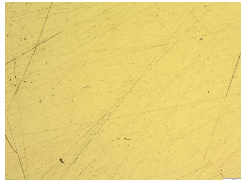
9:1 v/v MeCN to 2M HCl (aq) 7 Days at 50C HC-22, No corrosion
