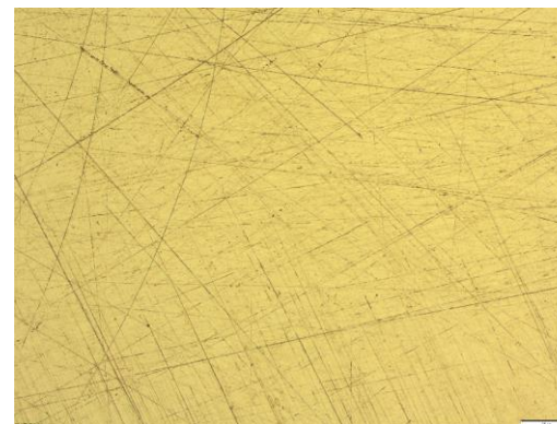
25C, 5x; No corrosion
